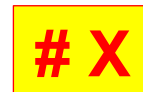
FIGURE 2 – PANEL-INTERIOR PLACARD (i.e., PLACARD TO IDENTIFY SPECIFIC SWITCHES/BREAKERS WITHIN THE SAME PANEL)
